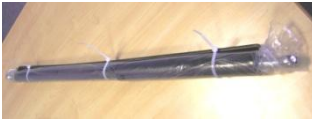
Fig #1 Gate Closer Cylinder assembled with retaining bar DO NOT REMOVE ZIP TIES UNTIL INSTALLED!
