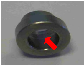
Grease Inside Stainless Steel Spacer (Fig 5)
