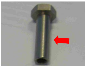
Grease Securing Shaft (Fig 4)
